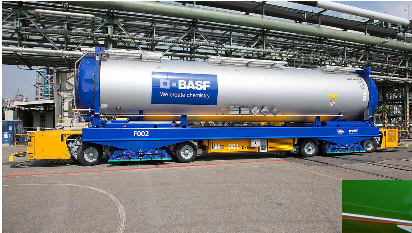
Automated Guided Vehicle (AGV), Tragrahmen und Tankcontainer B-TC Quelle: Pressefoto BASF
